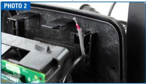
Make sure the EOG unit is not plugged in, connect the EOG unit's 2 wire leads to Relay 1 on the control valve. The black wire connects to **COM** and the red wire connects to **RLY1**. See **PHOTO 3** inset.
