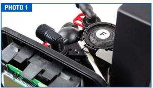
Unsnap the top of the control board bracket to expose the backplate and route the gray EOG wire through the hole as shown in **PHOTO 2**. Fit both wires into the wire chase and snap the bracket back into place. (Do Not Press on Control Board, use the bracket to snap into place.)
